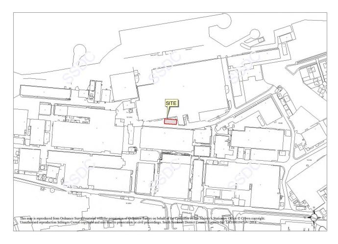
The site is located within the Augusta Westland site on Lysander Road. Building 147 is located in the centre of the site. It is a single storey building constructed of brick under a corrugated asbestos roof.
